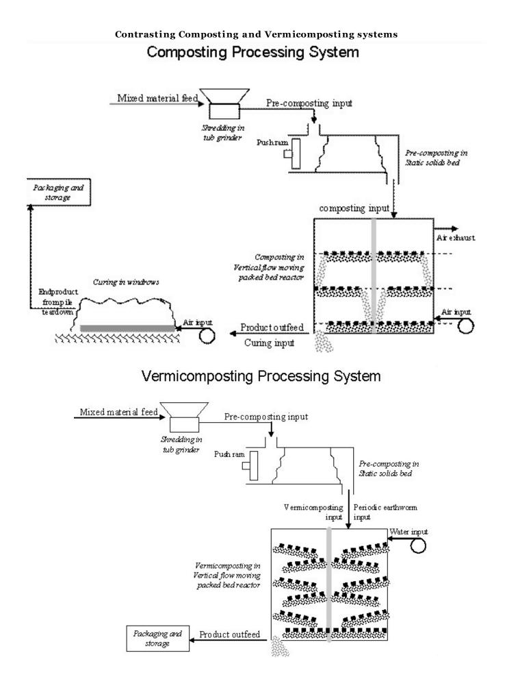
In both vermicomposting and composting systems, all cases waste needs to be transported with a payloader, shredded and mixed. This would reduce particle size and accelerate decomposition.
